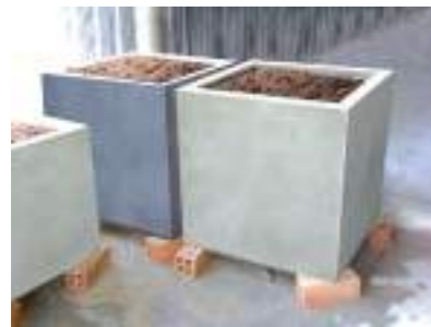
Durable body testing with full soil and water inside for testing strength ability of bottom, walls and corners
